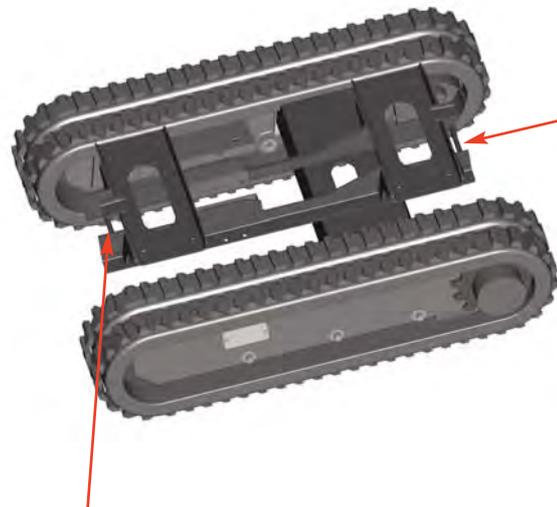
Tie down points located at front and back of chipper
