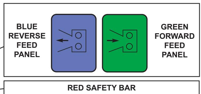
Do not rely on the red bar to keep the roller stationary if it is necessary to clear or touch the roller. Always switch off the machine and remove ignition key before approaching the roller.
