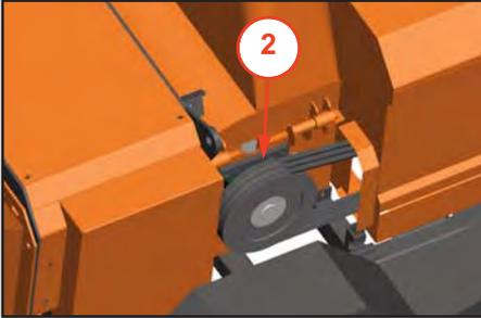
1. Remove the rotor housing guard, situated on the offside of the machine.
