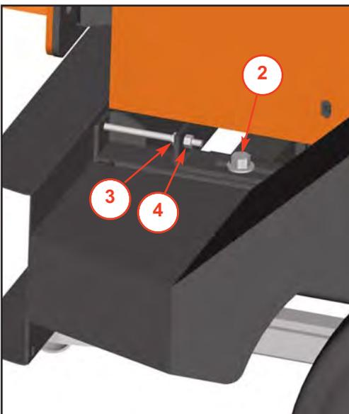
1. Remove the rotor housing guards, (as shown in diagram above).
