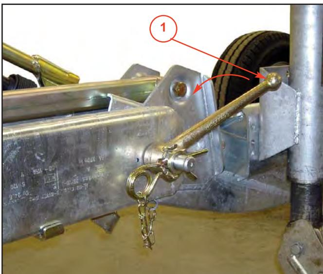
The preferred towing angle of any shredder is with the chassis level to the ground. The adjustable head has the ability to move between 300mm from the ground to 875mm giving an overall adjustment of 575mm.
