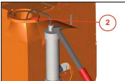
1. Remove the discharge tube.
